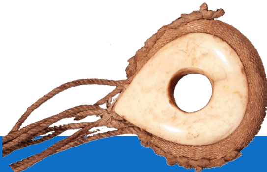
Whalebone Bullseye Fairlead, a device to guide line on a ship. Museum Collection.
